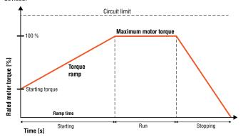
This function allows to start the motor when the initial torque is not sufficient to overcome friction forces; it transmits a high torque during the very first moments of the startup...
